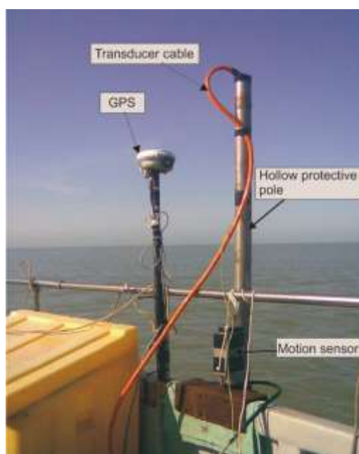
Figure 3L11: Motion sensor and GPS antenna attached to the pole holding the transducer source.
