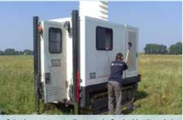
Seismic cone penetration tests in Doelpolder Noord. A sledge hammer and heavy beam were used to create acoustic waves (Image Courtesy RCMG).
