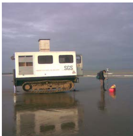
▲ Cone penetration testing on the beach at Raversijde (courtesy UGent).
