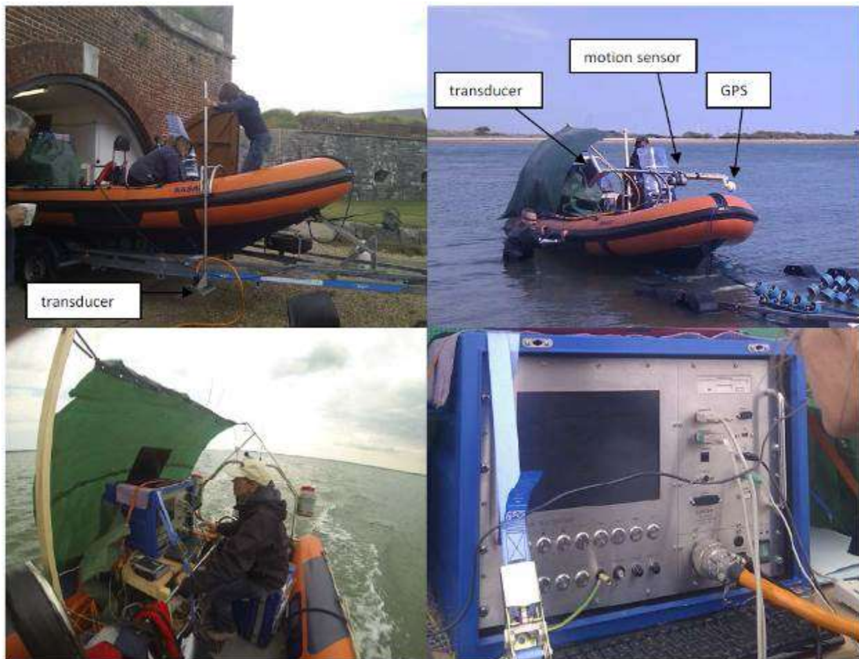
Figure 3D.53: Marine Seismic survey in Langstone Harbour. Upper left: Installation of the transducer pole onto the RIB. The pole is attached to a tilting system that fits over the inflatable hull. Upper right: transducer pole tilted horizontally during transit; GPS and motion sensor are on the right. Lower left: Data acquisition on board the RIB in Langstone Harbour. Lower right: close-up of the SES acquisition unit.
