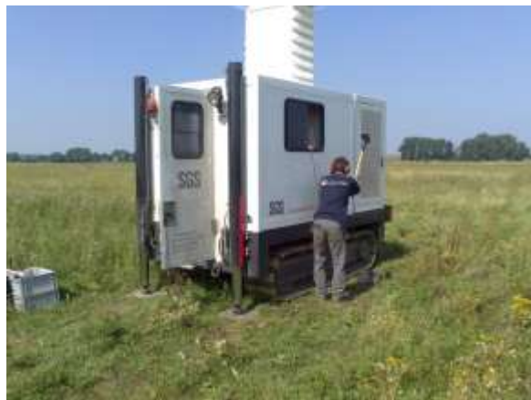
Figure 3M10: Left – CPT truck used for CPT measurements in the polder. A hammer blow is used to generate seismic waves. Right - Mobile CPT rig used for CPT measurements on the marsh. Due to a hidden gully the rig toppled over and had to be hauled out by a crane.
