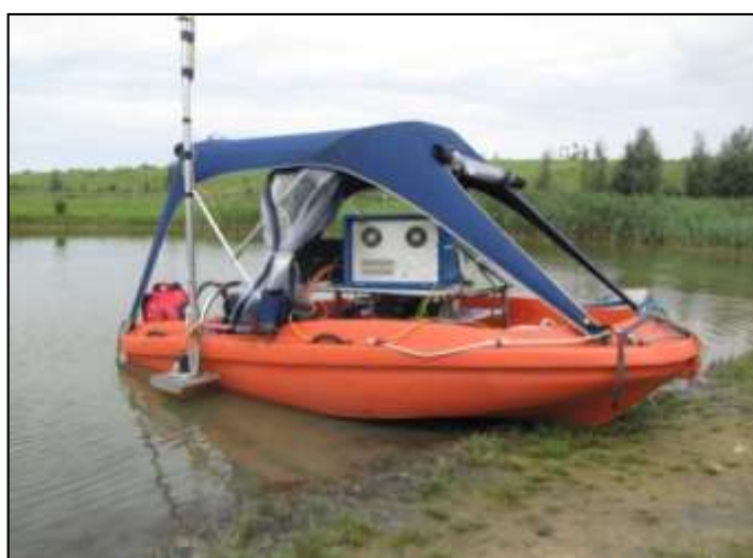
Figure 3M13: Left – seismic network on the Scheldt river (blue: intertidal; red: subtidal). Right – boat used for measurements on the inland creeks of Doelpolder-Noord.
