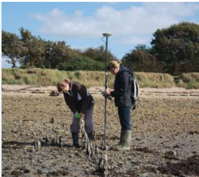
Figure 2.116. The RTK GPS system in use on a timber structure off Hayling Island
