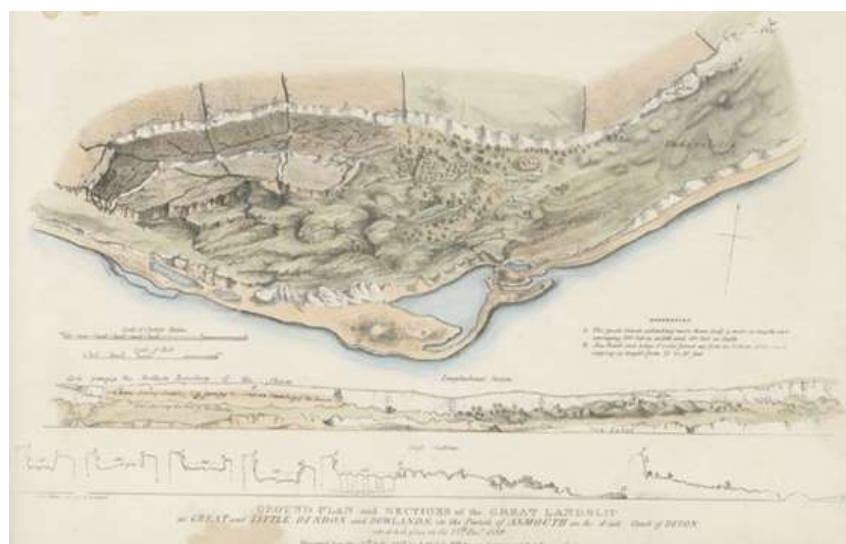
Figure 3E10: The area of the Bindon and Dowlands landslip was studied in detail and the geomorphology was mapped. Private Collection.
